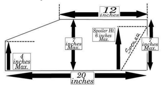
Modified spoilers may use maximum 2 side panels shaped like or similar to diagram template. Modifieds may use 2 maximum inside support braces shaped like or similar to diagram template.
