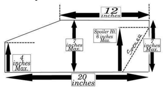
Modified spoilers may use maximum 2 side panels shaped like or similar to diagram template.
