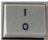
Switch the button to 'I' to turn on the transmitter, and 'O' to turn off the transmitter.
