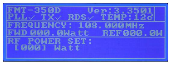
to increase the power or to decrease the power level. The power range is  $0^80/150/300/600$  Watts, depends on product model. The step is 1W for FMT-150D/350D/600D and 0.1W for FMT-80D. For quick power set, press and hold the button can increase or decrease the power continuously.
