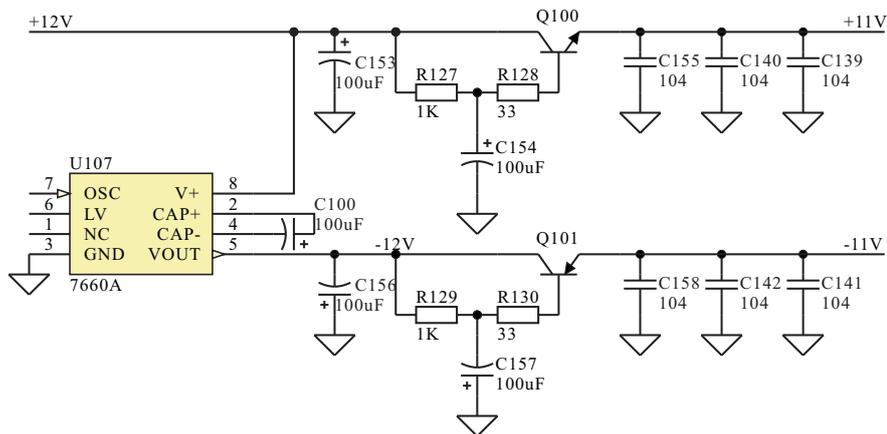
$\pm 11V$  voltage have two test point in the main board. show as below.
