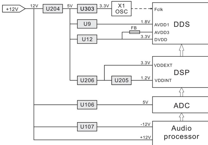
U107 performs supply voltage conversions from +12V to -12V, after these voltage are supply to operational amplifier via the filter. final voltage is about  $\pm 11V$ .
