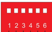
The toggle switch is use for set audio input impedance and pre-emphasis. Audio input impedance can set at 10KΩ or 600Ω. Pre-emphasis can be set at 25µs, 50µs, 75µs or OFF(flat). 25µs and 50µs can be combine to 75µs.
