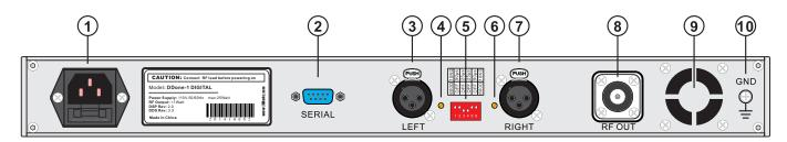
[1] MAINS Standard IEC connector for mains supply 110 or 230 V, +10/-15%
