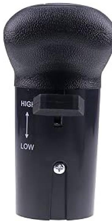
**SHIFTING FROM LOW TO HIGH GEARS, CONTINUE** WITH THE SAME CADANCE. **REMEMBER TO HIT** THE SPLITER WHILE IN 5<sup>TH</sup> **BEFORE YOU GO TO 6**<sup>TH</sup>.
