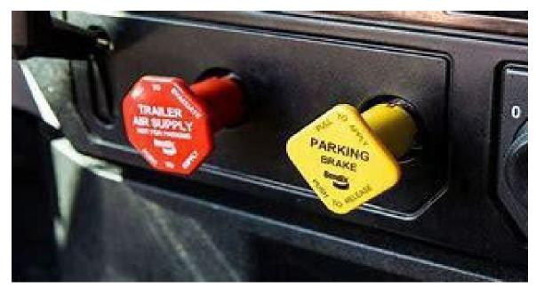
After the governor cuts off. Place the truck neutral, press and hold down your foot brake, turn the truck off, put key in accessory ,push in both valves, wait for air to stabilize. After initial loss of air, you should not lose more than 4 psi in one minute. Air stabilizes, then start your timer.
