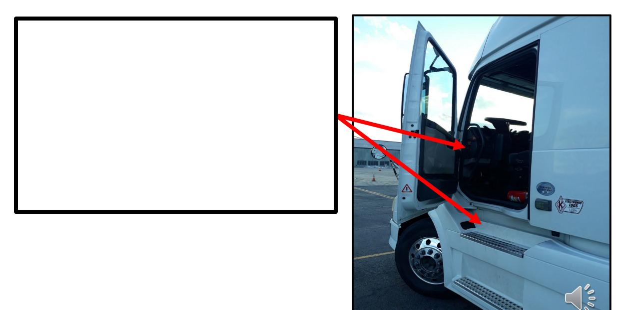
Pre- Trip begins with the in-cab inspection. Remember to always use 3 POINTS OF CONTACT
