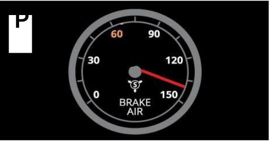
"Governor Cut off" Build air between 120 and 140 psi or governor cut off. After you start the vehicle build up air pressure and when governor kicks in, if it's within range it is working properly.
