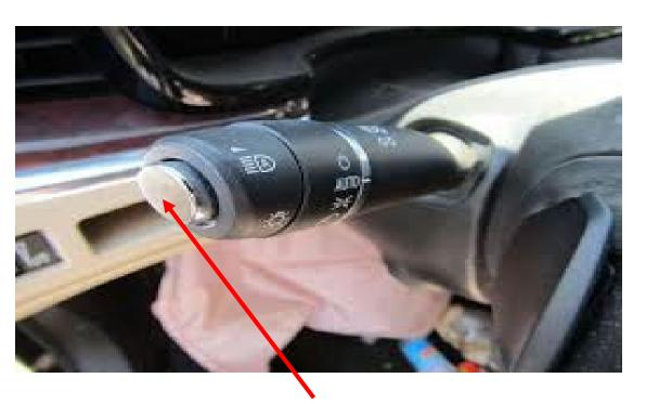
TURN SIGNAS, PULL BACK FOR HIGH BEAM, ALSO PUSH IN BUTTON FOR WIPERS AND WASHERS CHECK.
