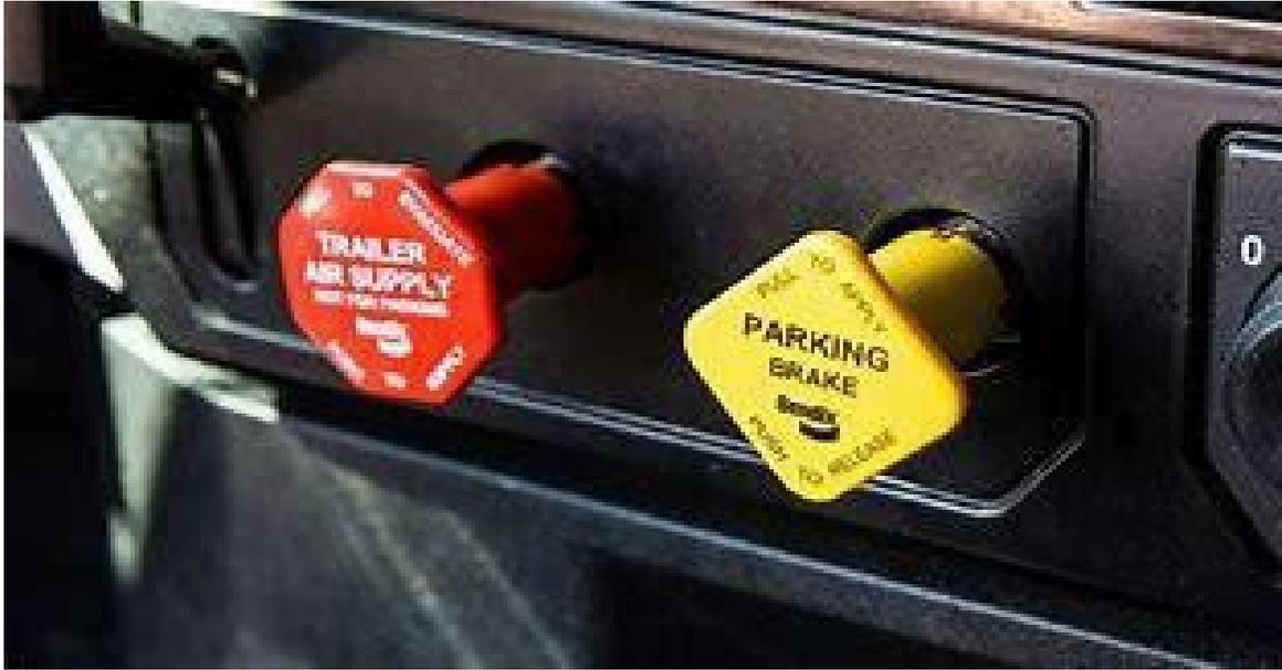
After the governor cuts off. Put truck in gear or neutral, press and hold down your foot brake, turn the truck off, put key in accessory, push in both valves, wait for air to stabilize. After initial loss of air, you should not lose more than 4 psi in one minute. Air stabilizes, then start your timer.
