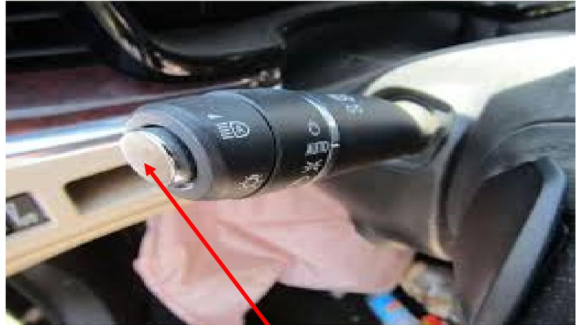
TURN SIGNALS, PULL BACK FOR HIGH BEAM, ALSO PUSH IN BUTTON FOR WIPERS AND WASHERS CHECK.
