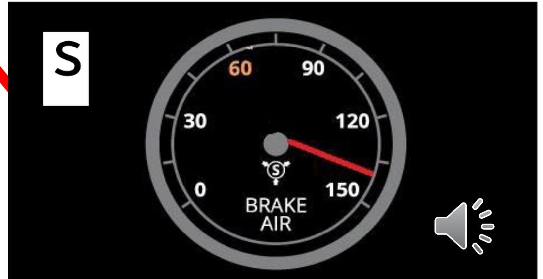
**"Governor Cut off" Build air between 120 and 140 psi or governor cut off. After you start the vehicle build up air pressure and when governor kicks in, if it's within range it is working properly.**
