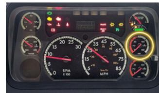
USED TO MEASURE TRAILER PSI
