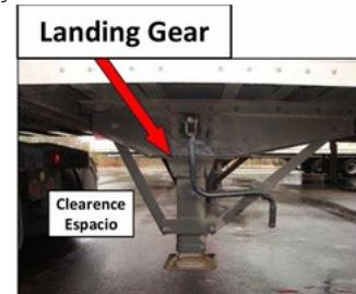
All Securely Mounted, Not broken, Not cracked
