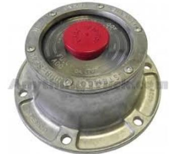
All Securely Mounted, Not broken, Not cracked All hardware are present and tight. They have no shiny thread or rust trails.
