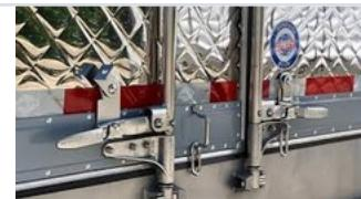
SECURELY MOUNTED, LOCKED POSITION
