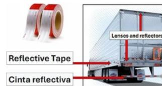
All Securely Mounted, Not broken, Not cracked All not missing, proper color clean and clear
