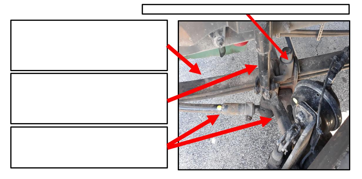
Air Bags (If equipped) Not cracked or leaking. Securely mounted.
