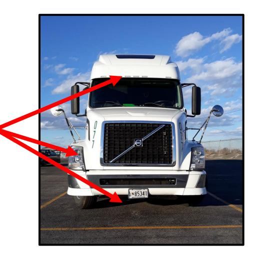
Take a step back and inspect to verify the vehicle is sitting level in the Front side to side. On the side from front to back.
