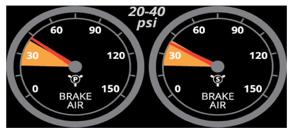
Safe start the vehicle and build up air pressure to at least (90psi).
