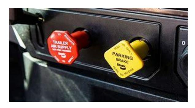
Put truck in gear, push in both valves, turn truck off and put key in accessory position.
