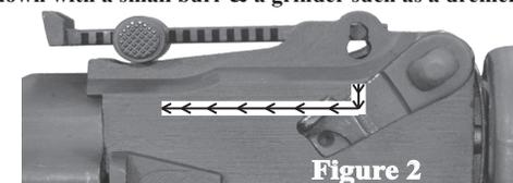
**Note:** A side view of the path the rear flip sight must travel to be removed (see figure 2).
