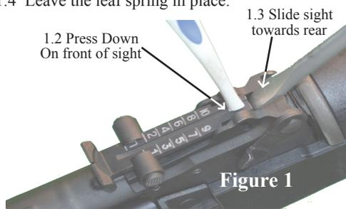
**Note:** Some SKS rifles have a pin that protrudes from the center of the retaining pin on original rear sight. This pin must be removed prior to being able to fully depress the rear sight. First try to tap it out with a very small punch & hammer. If that doesn’t work it will have to be ground down with a small burr & a grinder such as a dremel tool.
