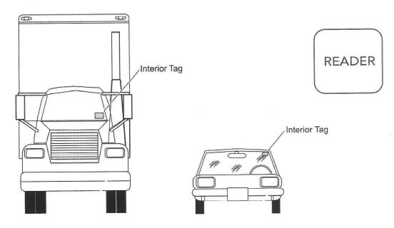
If the UHF reader antenna is installed to the right of the vehicle, optimal tag position is on the **right side** of the vehicle.
