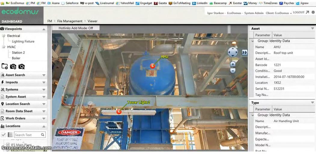
BIM Models Combined with Laser Scanned / Photo Imagery
