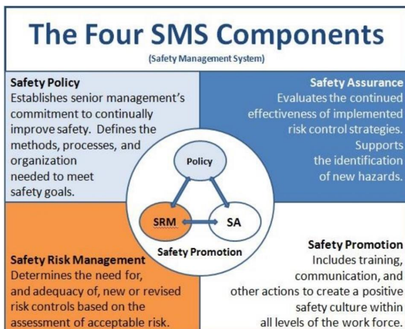
Figure C-1: SMS is comprised of four basic components described in this diagram from the FAA's AC 150/5200-37A.
