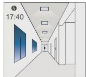
The light automatically turns on at 10% when natural light is insufficient (no motion).
