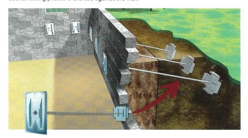
The Grip-Tite Wall Anchor system is a permanent, long-lasting solution for property owners facing issues with cracked, leaning, or bowed basement walls due to saturated and expansive soils along the exterior of the wall. This system provides a more cost-effective and less invasive alternative to complete wall replacement, ensuring stability and safety for the property.
