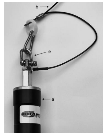
Plate 4. Transformer Electrical and Mechanical Connections.
