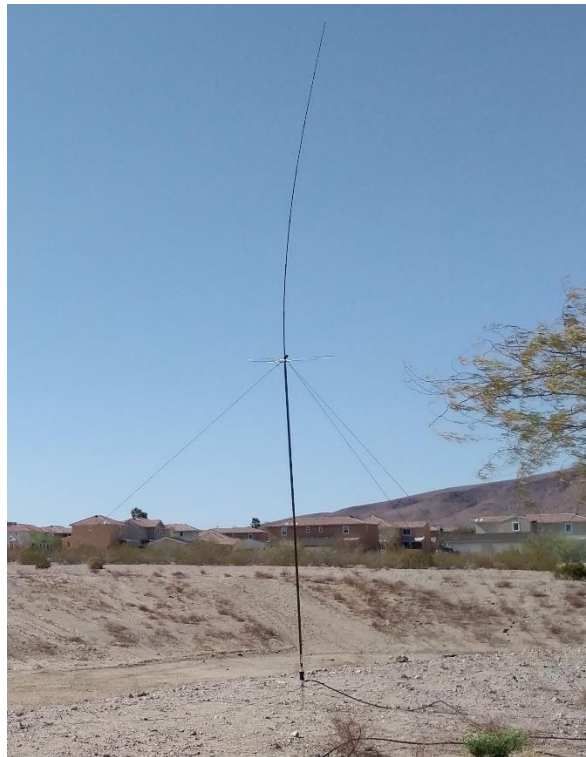
Figure 9 - Chameleon MPAS 2.0 with capacity hat in vertical configuration
