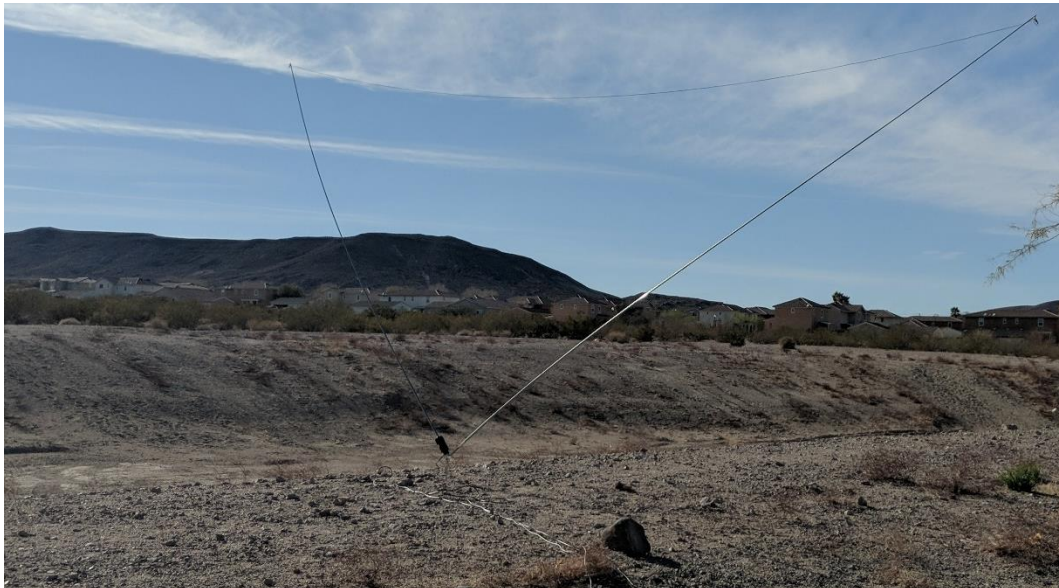
Figure 7 - Tactical Delta Loop ground spike mounted
