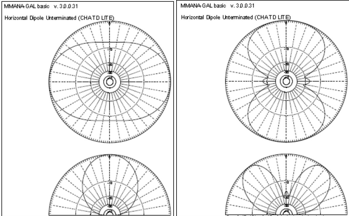
Figure 8. Horizontal; Dipole Far Field Plots, 7 (left) and 14 (right) MHz.
