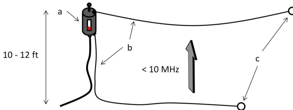
**Figure 6. Horizontal NVIS Configuration.**
