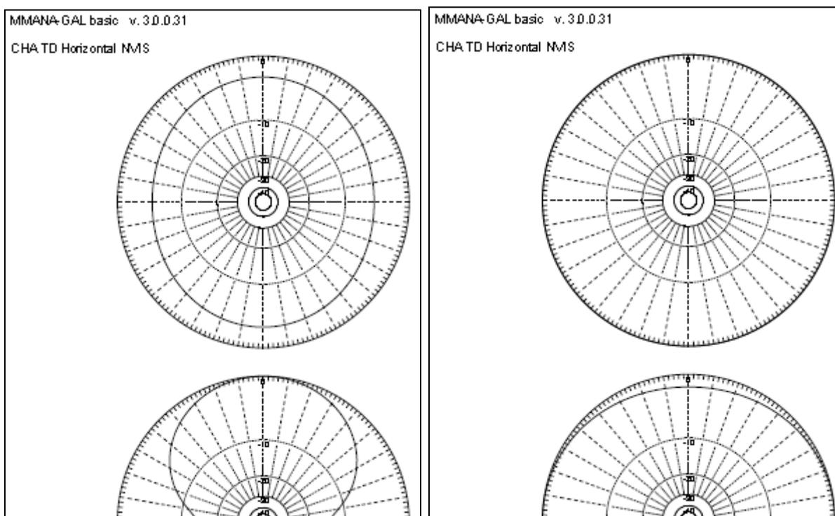
Figure 11. Horizontal NVIS Far Field Plots, 3.7 (left) and 7 (right) MHz.
