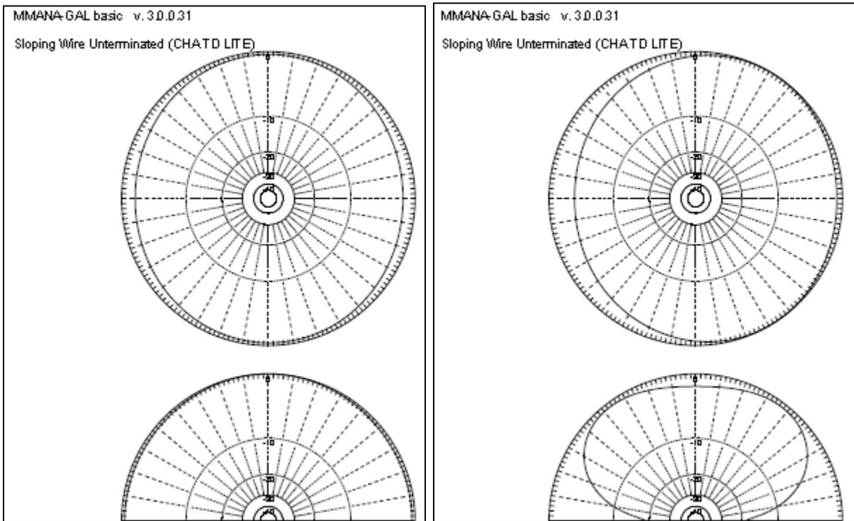
Figure 9. Sloping Wire Far Field Plots, 7 (left) and 14 (right) MHz.
