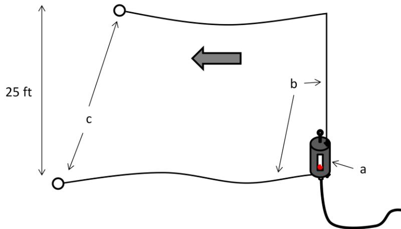
Figure 5. Inverted L Configuration.
