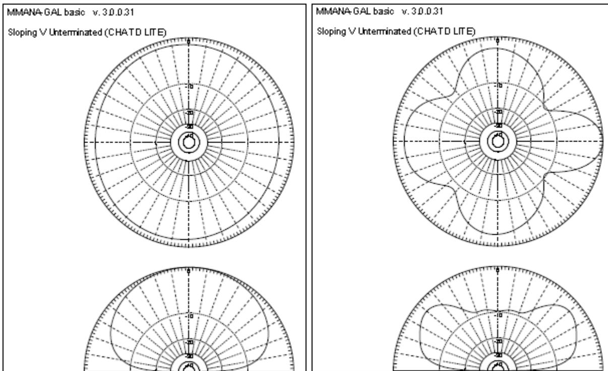
Figure 7. Sloping "V" Far Field Plots, 7 (left) and 21 (right) MHz.
