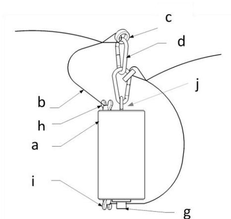
Figure 2. Matching Transformer Electrical and Mechanical Connections.
