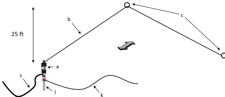
Figure 6. Inverted "V" Configuration.
