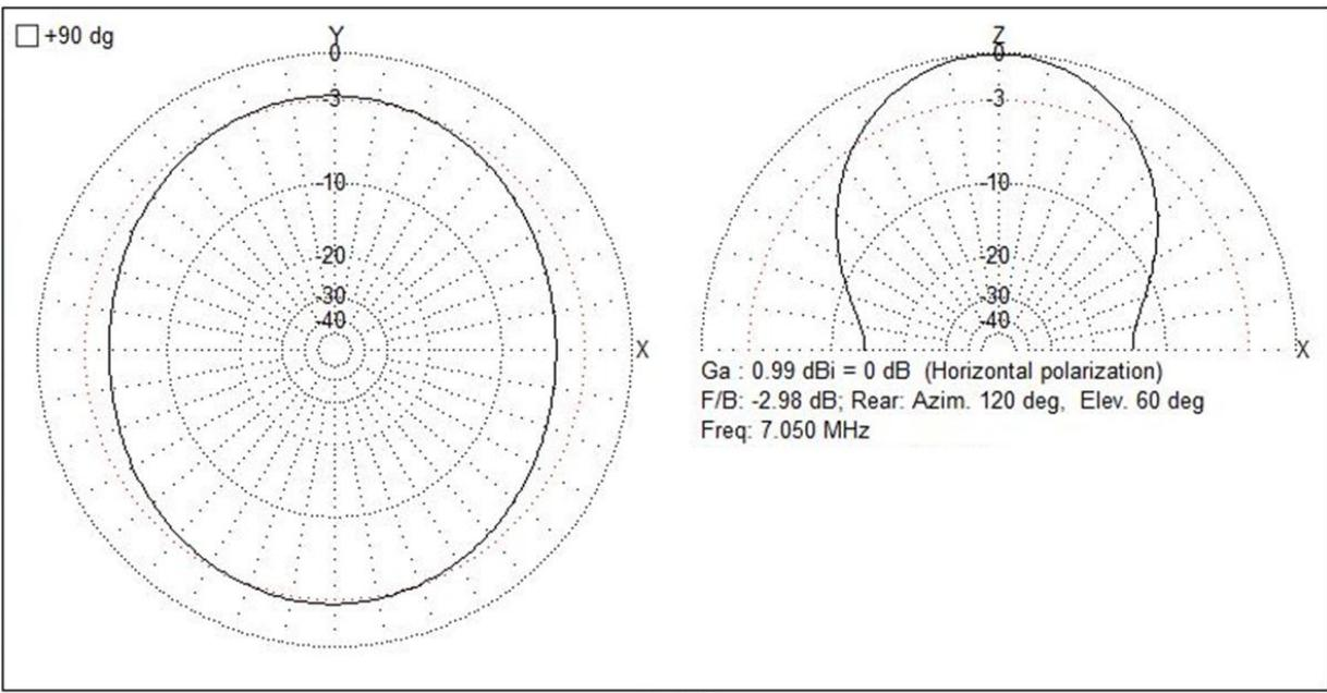
Figure 12. Horizontal NVIS Far Field Plot 7 MHz.
