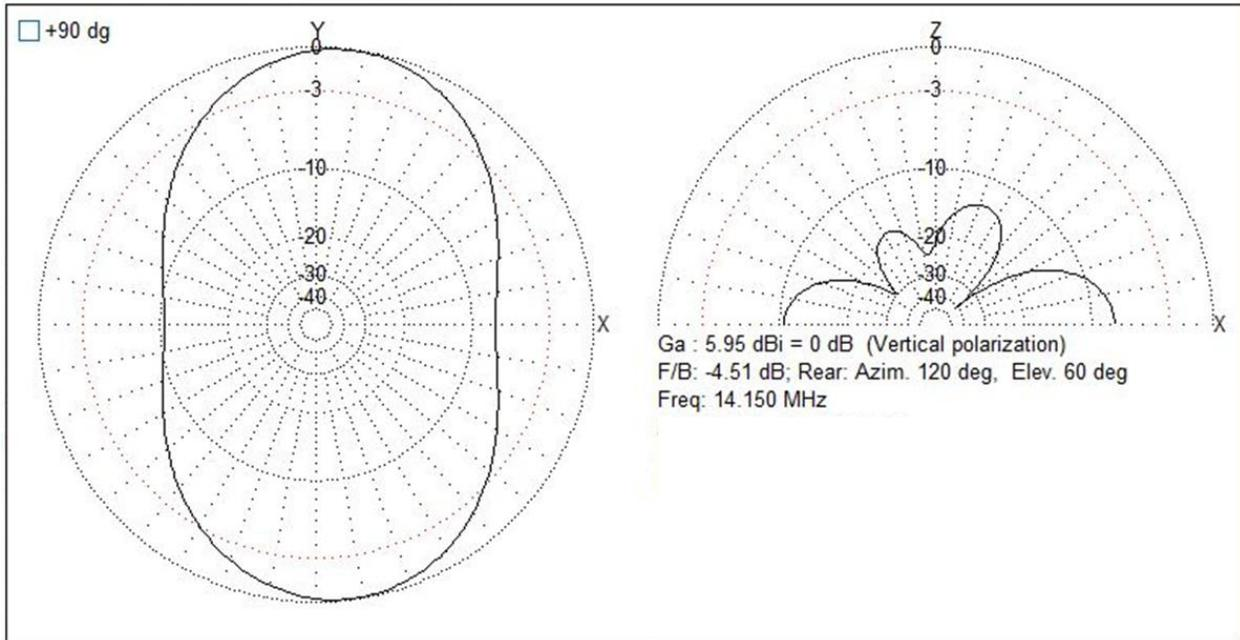
Figure 15. End-Fed Inverted "V" Far Field Plot 14 MHz.
