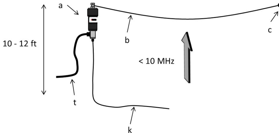
**Figure 3. Horizontal NVIS Configuration.**
