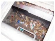
Debris removal efficiency was virtually 100%. The captured debris air-dried quickly and remained in a state of dryness. Sieve analysis of the sediment and grass seeds is shown in the following figure. USC collected water quality samples in the curb inlet and discharge, reporting removal efficiencies of various dissolved constituents shown in the table below.
