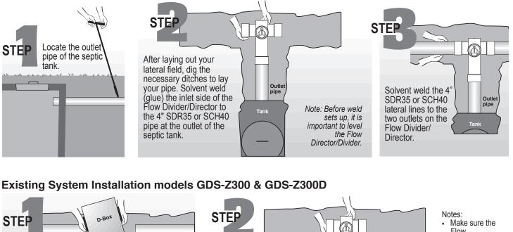
Solvent weld (glue) the inlet
