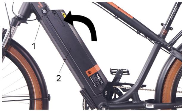
To reinsert the battery push the bottom of the battery (1) into the frame as far as it will go and then insert the top end of the battery into the frame until it clicks in place. You may then remove the key.
