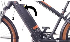
To pull out the battery, insert and turn the key. Hold the key in the unlock position (2) and then pull out battery (1).
