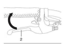
The right brake lever (2) controls the rear wheel
