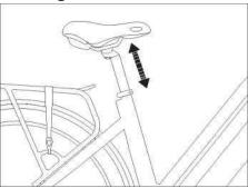
To ensure comfortable, fatigue-free and safe riding, the saddle and handlebar height should be adjusted to the riders body size. The saddle height is correct when the foot is resting on the pedal at the lowest position while the leg is not fully extended. The tips of the toes should be able touch the ground. Raising or lowering the seat to the height of the rider's hip, while they are standing on the ground next to the bike, is a good starting point.
