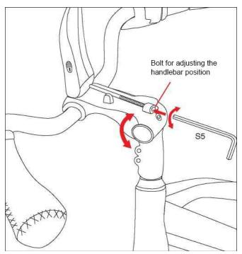
3. Move the handlebar up or down to the desired position. If it is too loose or too tight, please adjust the screw on the handlebars.
