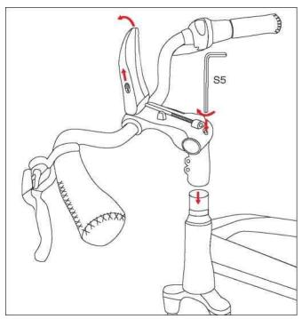
1. Install the handlebars as shown and tighten the upper screw.
