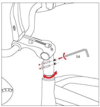
2. Adjust the handlebar to the desired position and tighten the screws on the right side.
