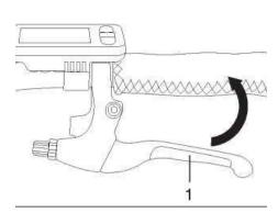
The left brake lever (1) controls the front brake
