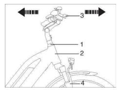
The front fork (4) must not become stuck in the steering position and must swing easily in both directions.
