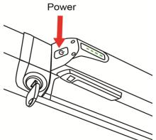
The 4 LEDs located on the top of the battery indicate the charge level.
