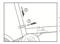
Grab the seat so it doesn't mistakenly drop to the ground and loosen the seat post clamp.
