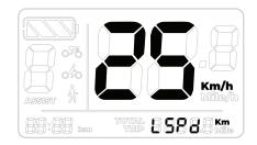
Press the power button **b** to save and go to set backlight setting.
