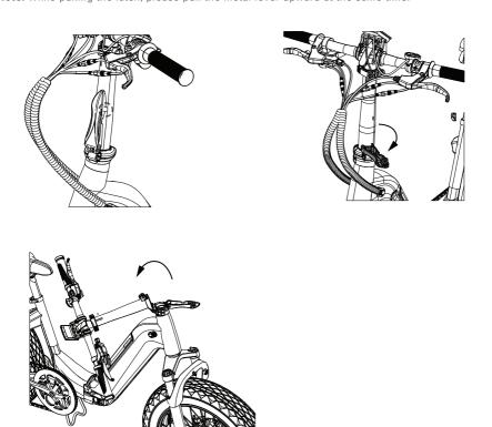
4. Holding the latch lock up, use your other hand to open the latch by pulling it away from the frame, folding the rear wheel/section towards the other wheel and use the stand under the frame as needed.
