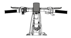
**Step 5.** Release the clamp under the handlebar, pull the handlebar up or push it down to adjust height as your desired, then close the clamp to secure handlebar in place.
