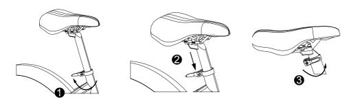
**3.** Release the latch by pulling it down away from the stem, then slide to the left side (see below illustrations) then fold the stem down.
