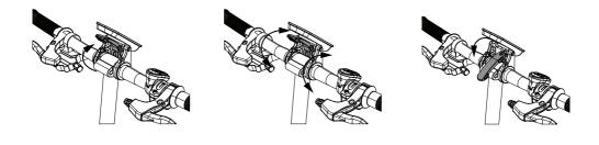
**Step 4.** Use a 3mm hex key to loosen display screws. Then install display onto handlebar using 3mm hex key and tighten screws.
