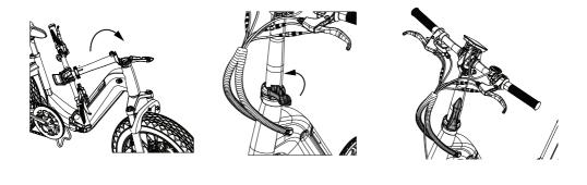
**Step 3.** Stand in front of the bike and clamp front wheel with both legs, adjusting handle bar angle to make sure the bike is straight in line. Sit on the saddle, adjust the handlebar to comfortable angle, and close the handlebar clamp to tighten the handlebar.
