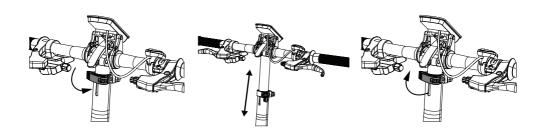
**Step 6.** Open the clamp under the seat post,set it to a height which fifits for the rider then close the clamp to secure the seat in place.
