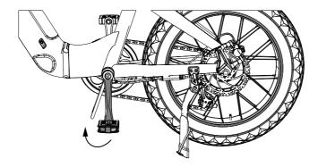
**Step 8.** Remove motor protector and put on the motor protection guard on both sides of back wheel. Install motor protection guard on both sides of back wheel.
