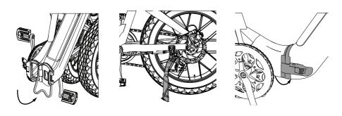
Step 2. -Pull the stem upright and fold the latch up to close it.
