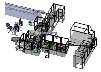
Assembly tolerances up to 0.05mm are achieved well within the required 1.3s cycle time.
