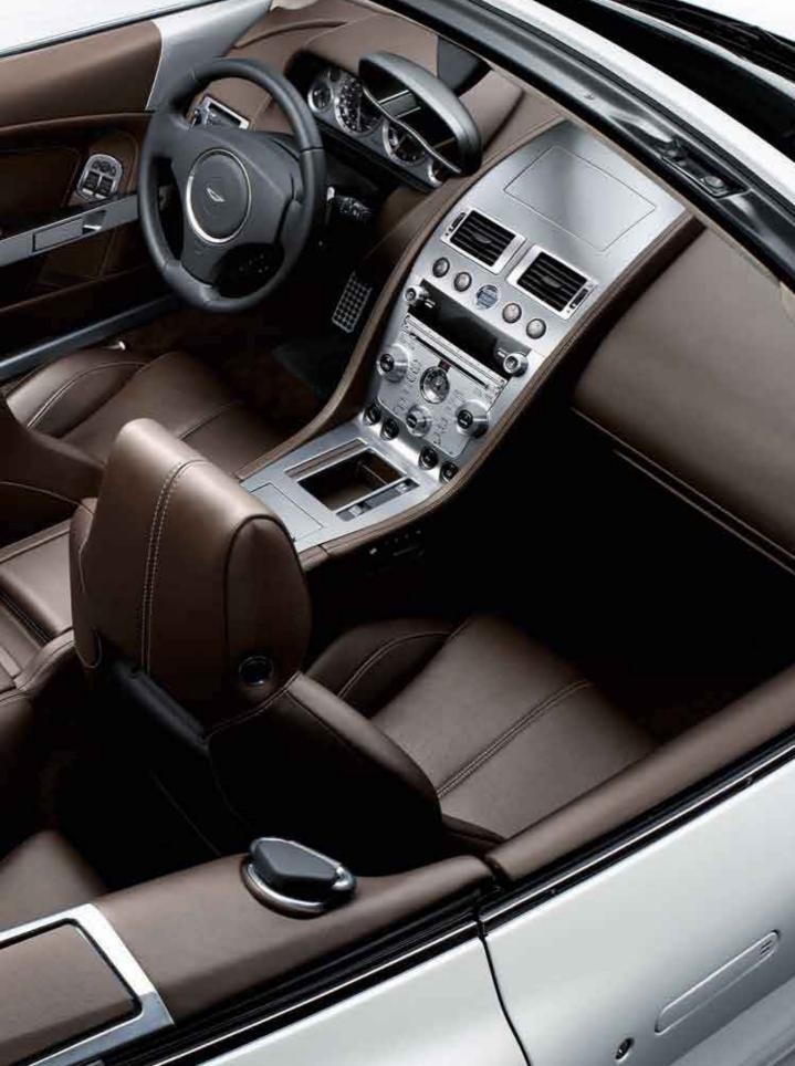
All controls are within easy reach. The highly intuitive 'Touchtronic 2' transmission is operated via simple, dashboard-mounted buttons, flanking the docking station for the ECU. A combination of solid aluminium dials and chromed buttons operate the DB9's audio systems, Bluetooth telephony and hard-disk based navigation, while a classic analogue clock is placed at the heart of the console.
