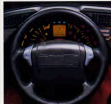
The new-for-1990 Supplemental Inflatable Restraint system (air bag) is located in the hub of the steering wheel. The S.I.R. is designed to provide added protection to the driver in the event that your Corvette is involved in a moderate to severe frontal impact. For maximum protection in frontal and all other collisions, both driver and passenger should be properly restrained with safety belts.
