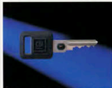
Corvette ZR-1 features PASS-Key®, the electronic anti-theft system that has proven itself the most effective theft deterrent Chevrolet has ever offered. PASS-Key is a special ignition system utilizing a module with a resistor decoder and an ignition key with a pellet of specified resistance. Vital systems are deactivated when you lock the ignition and can only be reengaged with your special PASS-Key ignition key. An anti-theft horn alarm is also standard on Corvette ZR-1.
