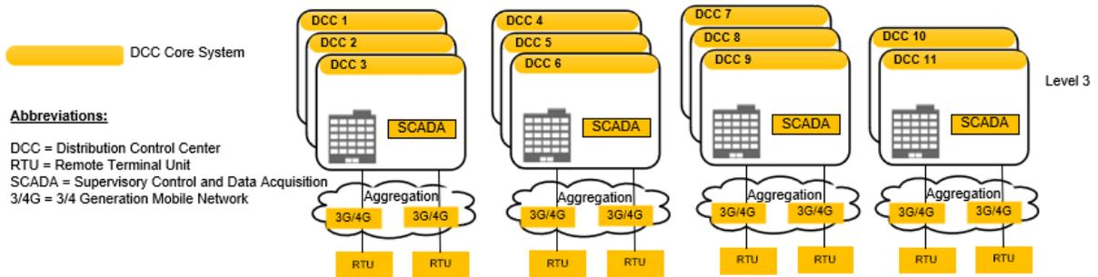
**FIGURE 32: SIEMENS SOLUTION OVERVIEW**
