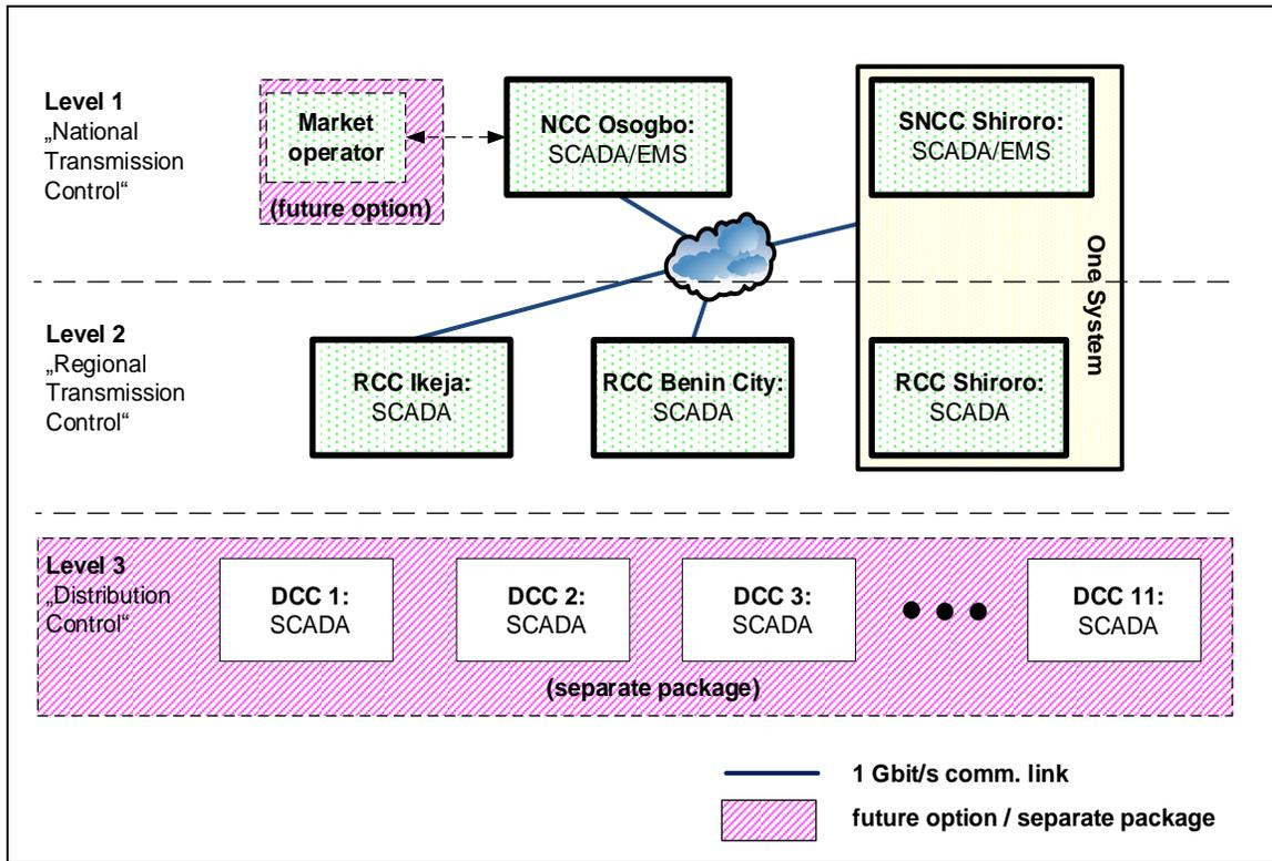
FIGURE 19: OVERALL ARCHITECTURE OF THE DRAFTED SCADA/EMS SOLUTION
