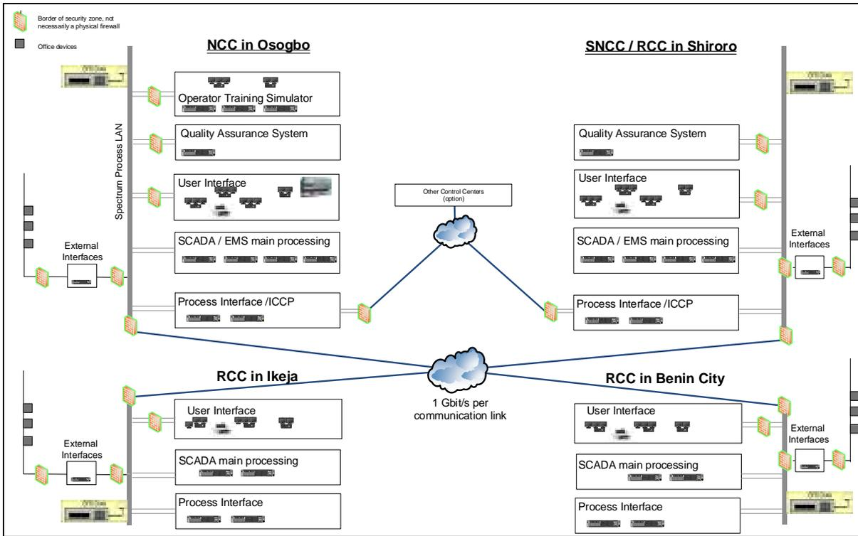
**FIGURE 20: DETAILED ARCHITECTURE OF THE DRAFTED SCADA/EMS SOLUTION**
