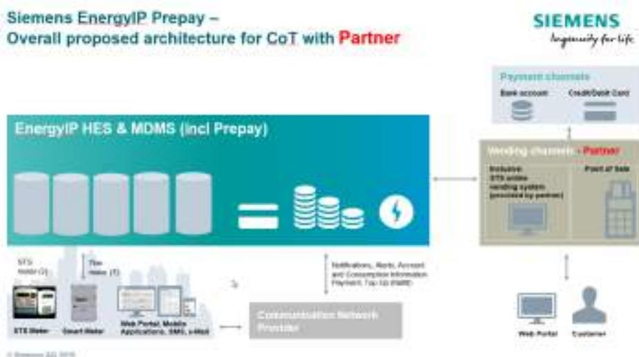
FIGURE 30 – MAJOR INTERFACES BETWEEN ENERGYIP PLATFORM AND THE ON-LINE VENDING PLATFORM
