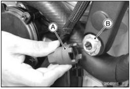
Using the Hexagon Wrench, turn the adjusting collars [A] counterclockwise to make the gap between the engine and adjusting collar.
