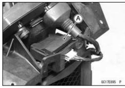
Oxygen Sensor [A] (Equipped Models)
