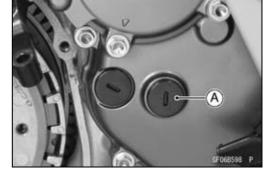
• Using a wrench on the starter clutch bolt, turn the crankshaft clockwise until the clutch stopper bolts [A] reaches the position as shown.
