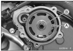
Remove: Starter Clutch Cover Bolts [A] Starter Clutch Cover [B]
