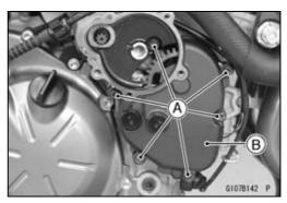
• Remove the idle gear (starter clutch side) [A] with the shaft [B].
