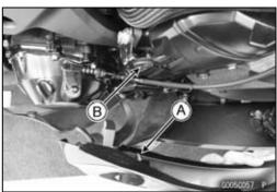
• For right lower fairing installation, insert the hole [A] into the projection [B] on the rear lower fairing.
