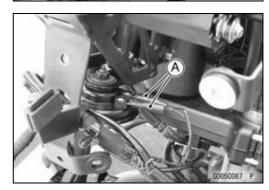
Remove: Bolts [A] Windshield Bracket Assembly [B]
