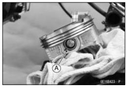
• Using the piston pin puller assembly [A], remove the piston pins.
