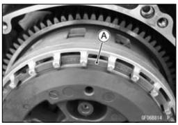
• Be sure to install the spring seats [A] on the clutch pressure plate.
