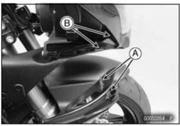
• Insert the hooks [A] into the slots [B] on the lower fairing (both sides).
