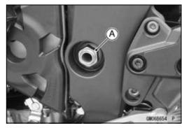
• Using the swingarm pivot nut wrench [A], loosen the swingarm pivot adjusting collar locknut [B].
