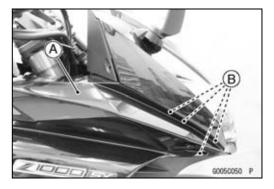
• Disconnect the turn signal light lead connector [A] (both sides).
