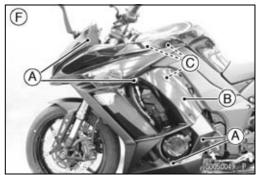
• Pull the lower fairing [A] rearward to clear the hooks [B], and remove the lower fairing by moving it downward (both sides).
