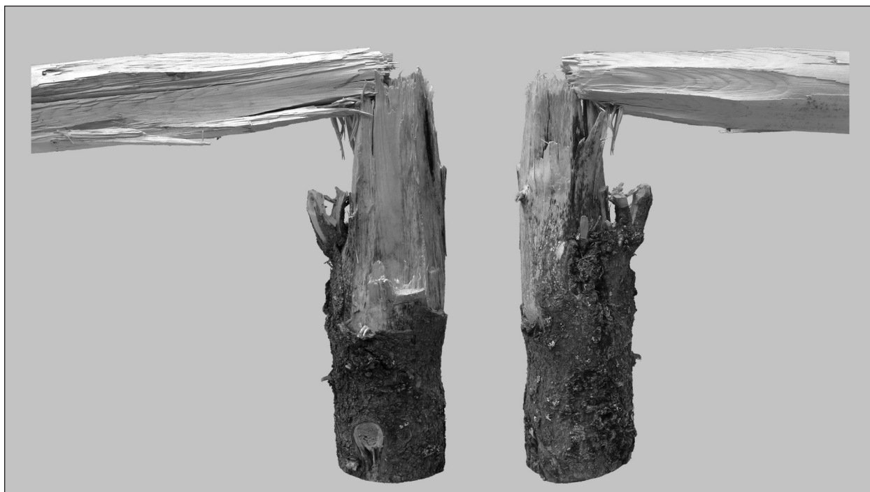
Figure 11: Detailed view of Experiment 1 stump and log. The height of the stump is 53 cm.
