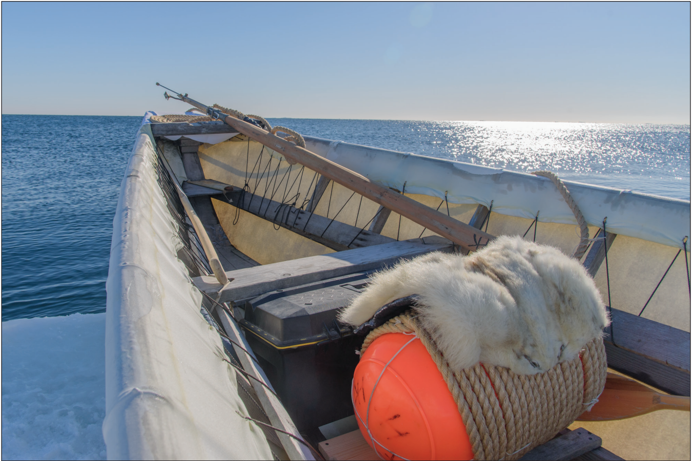
Figure 9. Nylon skin umiaq. Ballistic nylon with waterproof coating. April 26, 2017. Photo by the author.
