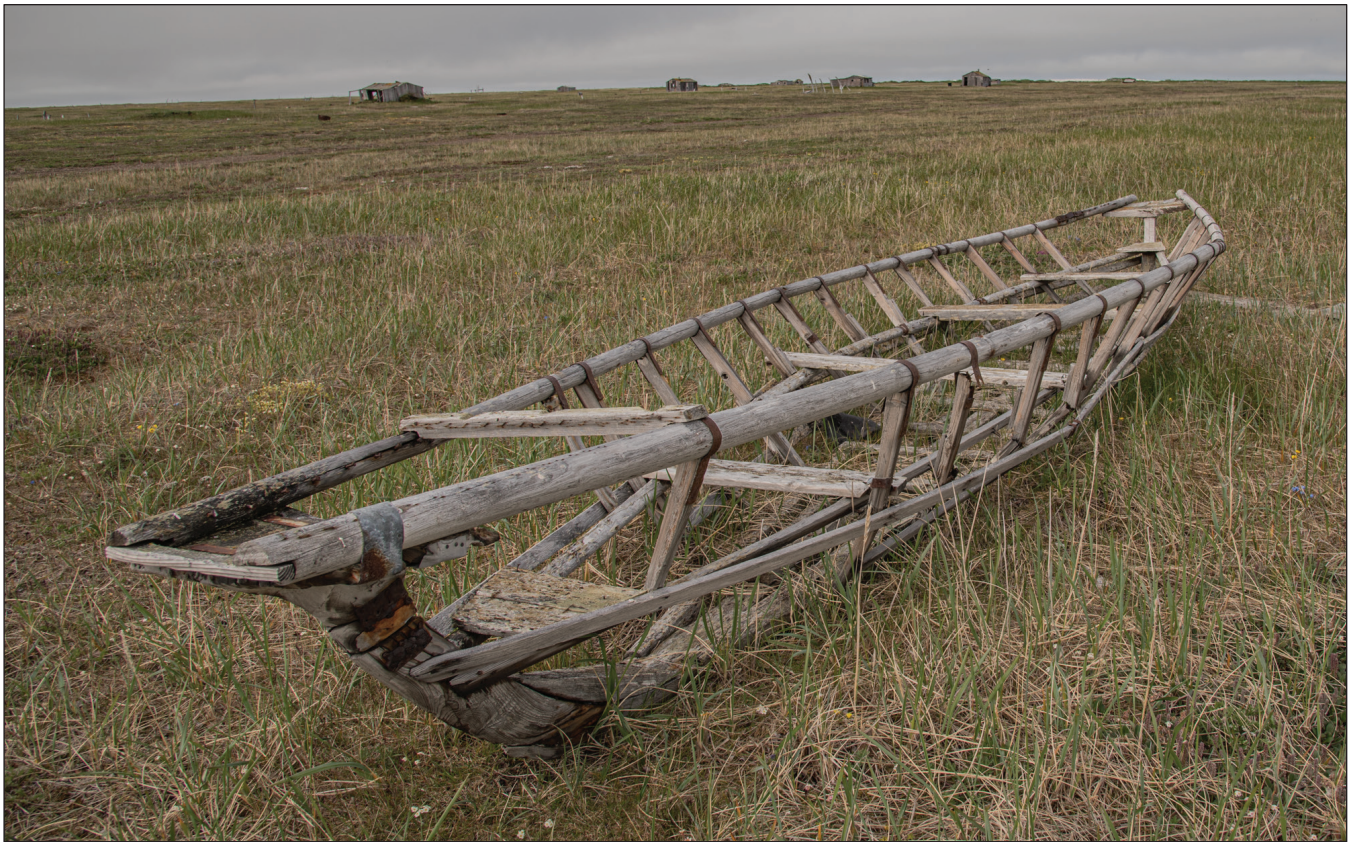
Figure 1. An umiaq frame using many metal parts that was built before the 1970s. July 11, 2021. Photo by the author.
