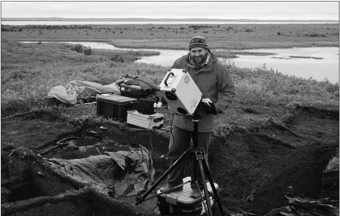
Figure 3. Using the Minolta laser scanner to capture an image of House 3.
