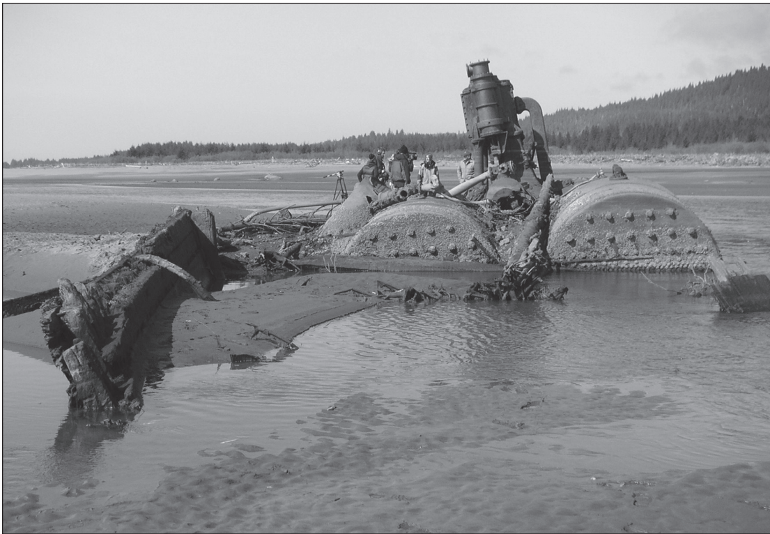
Figure 5. A view of the SS Portland wreckage from bow to stern, showing the double Scotch boilers and engine. A portion of starboard hull is visible. Photo by Dave McMahan.
