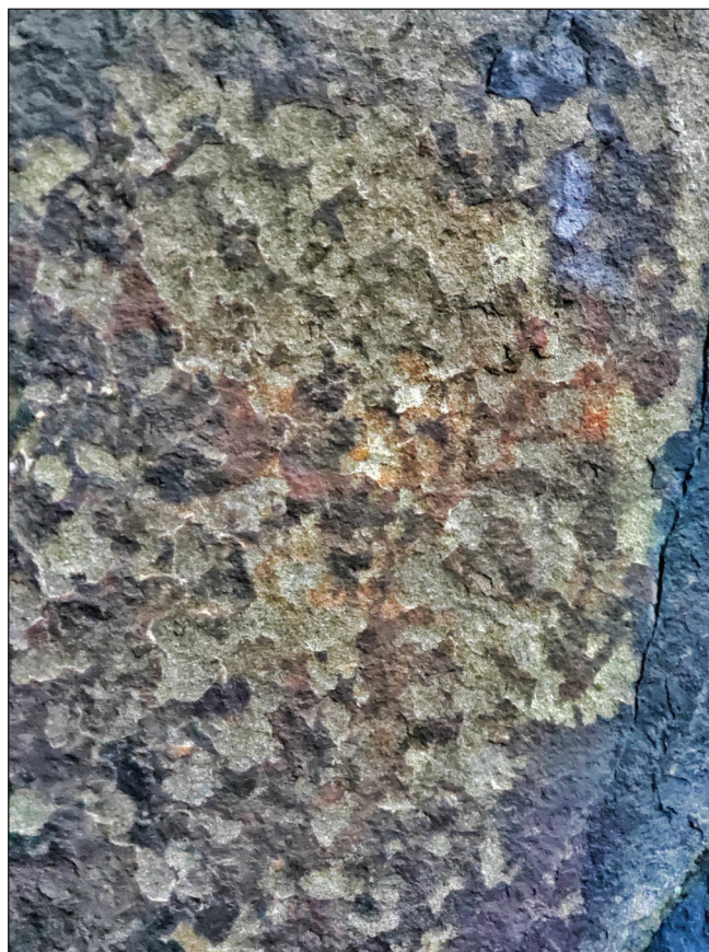
Figure 3. Image showing spalling and exfoliation of the rock surface.
