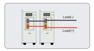
After parallel connection, the capacity of the battery system will be doubled according to the number of batteries you connect. E.g. If two 25. 6V 300Ahbatteries are connected in parallel, the battery system will be 24V(25.6V)600Ah.
