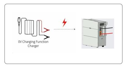
The charger can charge the battery starting from 0V.
