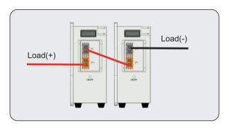
After series connection, the voltage of the battery system will be doubled according to the number of batteries you connect. E.g. If two 25.6V 300 Ah batteries are connected in series, the battery system will be 48V(51.2V) 300 Ah.
