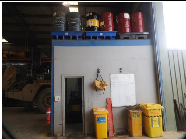
Photo 3: Self-bunded pallets with stored 205L drums above active area in the workshop. Spill kits are stored outside (1021B_0014)
