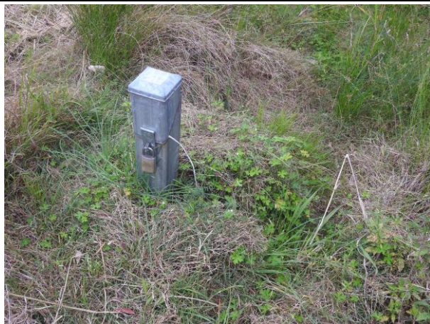
Photo 27: Piezometer monument for MW2 – not appropriately numbered (1021B_0082)
