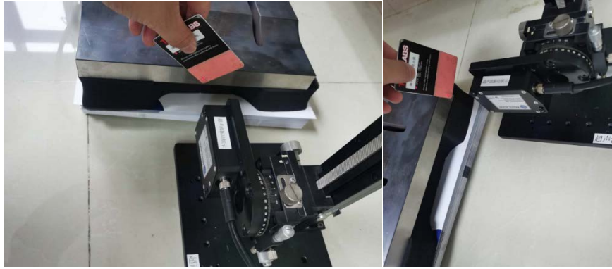
Fig. 3: Testing setup for 15KHz transducer
