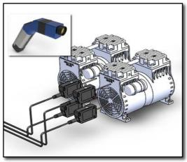
Motor Vibration Testing (Permanent installation or handheld device)
