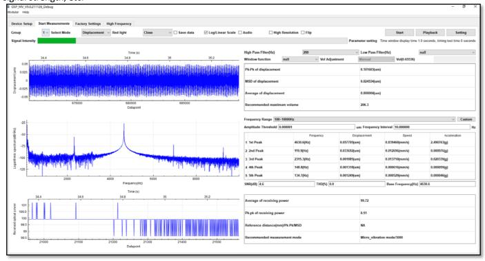
Option 2: DLL+LabView based testing GUI, suitable for testing oriented customization.
