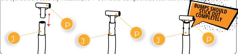
Insert the fiberglass stick trough the designed area in the safety net and connect it to the T-Connector.
