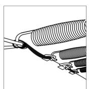
Cover the spring frame with the soft padding Frame Cover (A). Secure the padding parts together using the Velcro on each side, and tie the straps located underneath. Lay down the Frame Cover (A)so all the springs are covered. It should be fitted like a shower cap.
