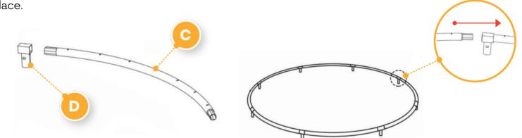
Two people will be necessary at this point to install the trampoline. One person lifts up the circle frame, while the other lifts the W shaped leg tubes to a standing (vertical) position and inserts the Steel T-Connectors (D) into a W-Shaped Leg tube. Ensure the locking holes are aligned.
