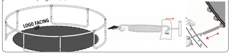
Start installing the springs in an X shape. The tension needs to be distributed evenly for the net to be installed correctly. Gently tap down against the spring if the hook is not completely in the hole. Springs will create high levels of tension when assembled. Please take care not to pinch your fingers.
