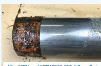
After 1000 hrs of ASTM B117-18 Salt Spray Test
