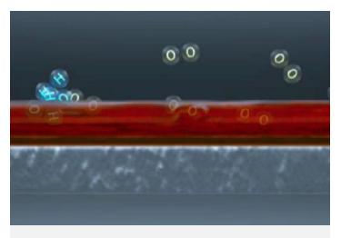
S2S PLID products displace oxygen and water to form a dielectric barrier protecting the metal from rust and corrosion.
